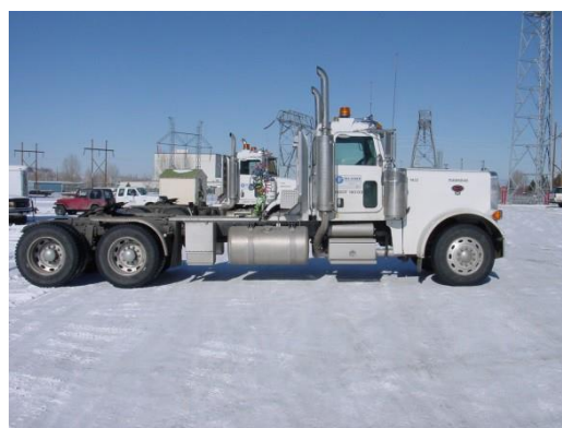
Heavy haul tractor: 8 feet wide, 18 – 25 feet length, and weight 8 – 12 tons.
