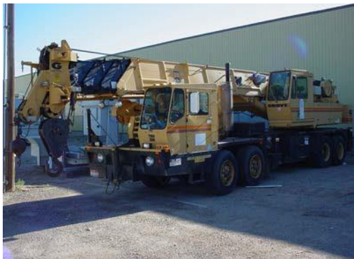
Crane: 8 – 10 feet wide, 30 – 70 feet length, weight 20 – 35 tons.
