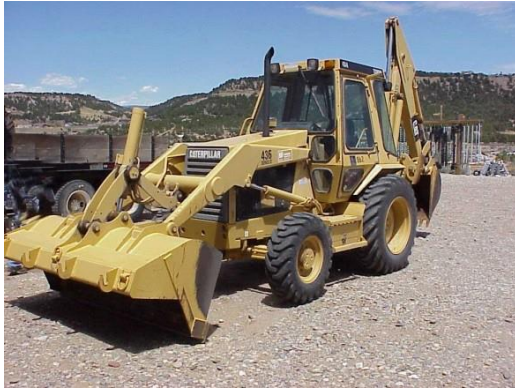
Backhoe: 8 feet wide, 15-20 feet length, and weight 10-15 tons.
