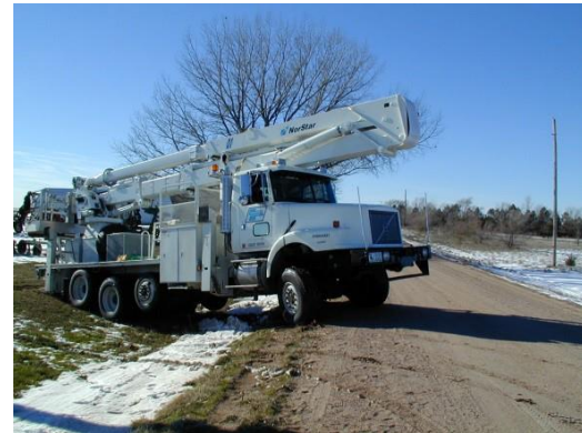
Bucket truck: 8 feet wide and 15 – 25 feet length.
