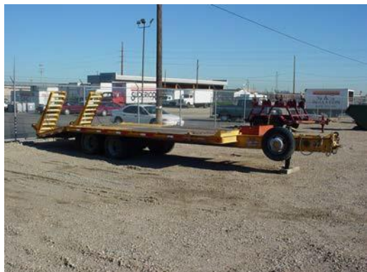
Equipment trailer: 10 – 12 feet wide and 20 – 40 feet length.
