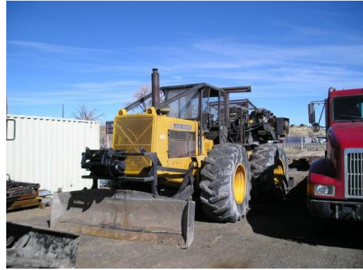
Brink skidder/Dozer: 8 – 12 feet wide, 15 - 25 feet length, and weight 15-30 tons.
