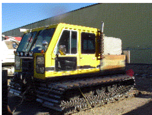
Snowcat or Linetrac: 8 – 10 feet wide, 20 feet length, and weight 15 – 30 tons.
