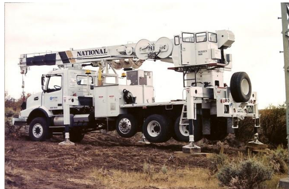
Digger derrick: 8 – 10 feet wide, 30 – 40 feet length, and weight 25 – 30 tons.
