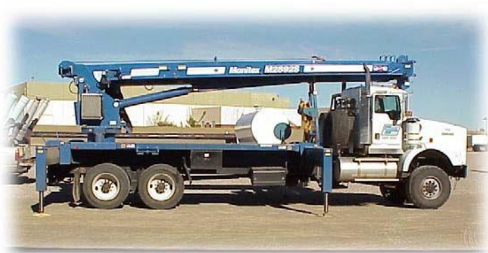
Boom truck: 8 – 10 feet wide, 30 – 45 feet length, and weight 30 – 40 tons.
